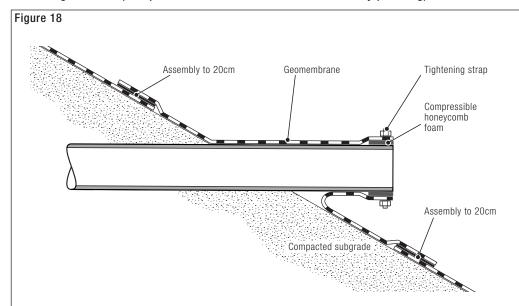
7.6.3 Connection to pipe, with or without pipe penetration into concrete structure for basin containing effluents (irrespective of whether or not environmentally polluting)
