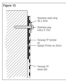
**Reminder 3:** The design must take into consideration the chemical aggressiveness of the fluid or its viscous or particle content, and so determine the method of protection to be provided by the mechanical fixings:
