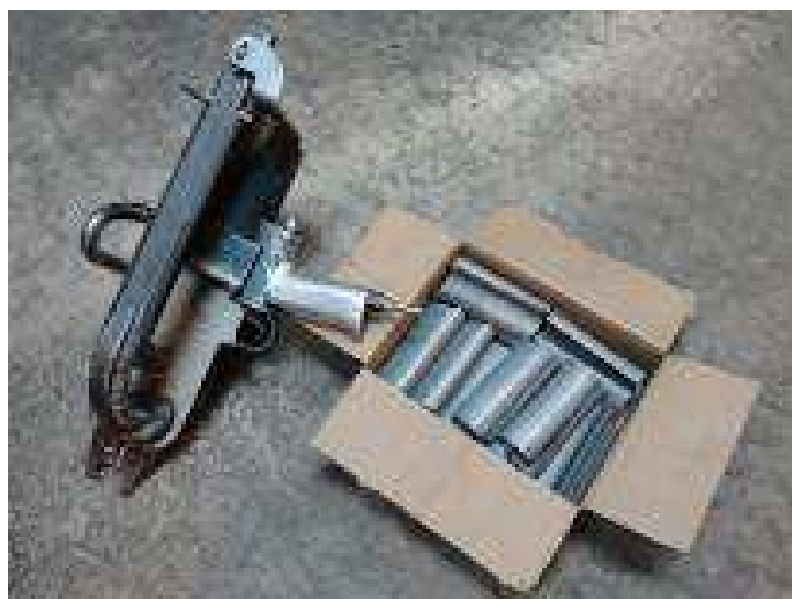
Above a Pneumatic Spenax installation tool, with a box of Spenax rings (1,600 rings/box)
