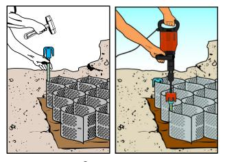
Figure 5 ATRA® Anchor Installation Methods
