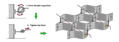
Figure 13 Termination of Integral Tendons
