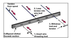
Figure 11 Threading Tendons
