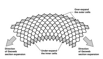
Figure 7 Curved Expansion of Section
