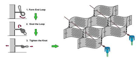
Figure 14 End Anchorage of Tendons
