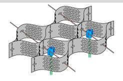
Figure 15 Internal Anchors
