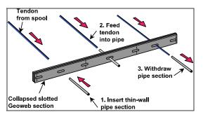
Figure 12 Use of Guide Tubes
