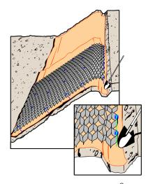
Figure 4 Placement of Geoweb® Section
