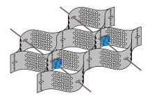
Figure 18 ATRA® Restraint Clips
