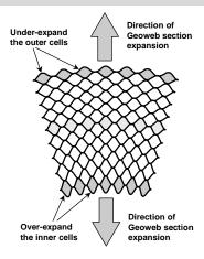
Figure 8 Tapered Expansion of Section
