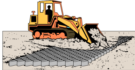
Figure 14 Fill Placement with Loader
