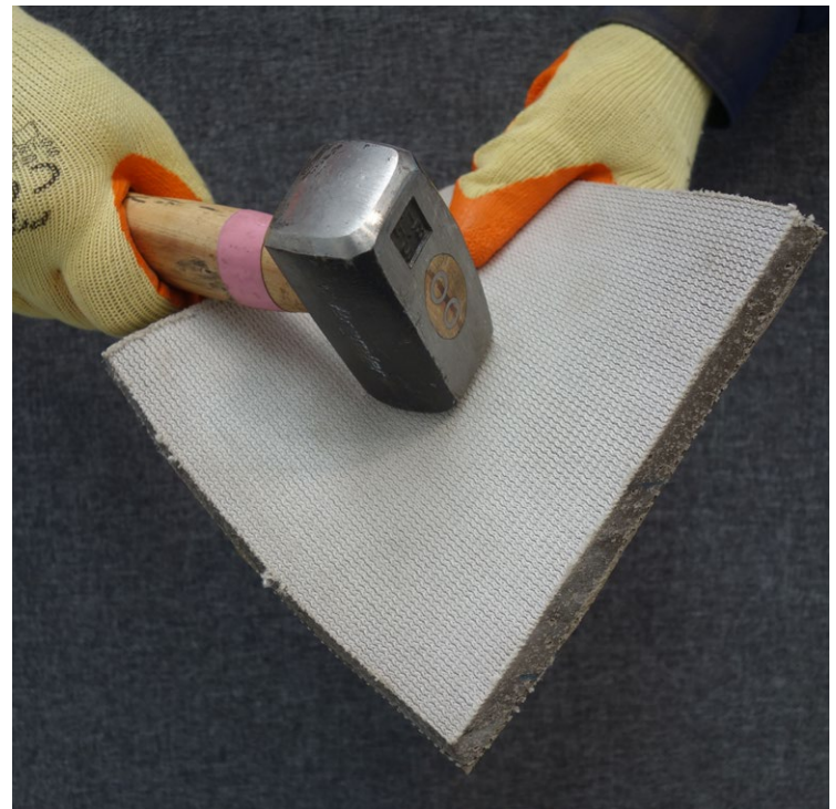
Figure 1. The change of GCCM properties from flexible to rigid on curing means that when assessing GCCM properties, appropriate test methods should be used to determine the cured, in-service GCCM cementitious layer performance.
