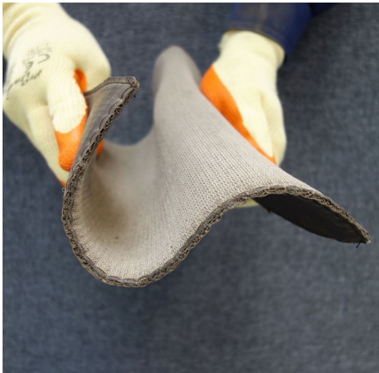
Figure 1. The change of GCCM properties from flexible to rigid on curing means that when assessing GCCM properties, appropriate test methods should be used to determine the cured, in-service GCCM cementitious layer performance.
