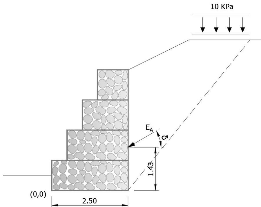
Figure 67 – Point of application | Active Thrust
