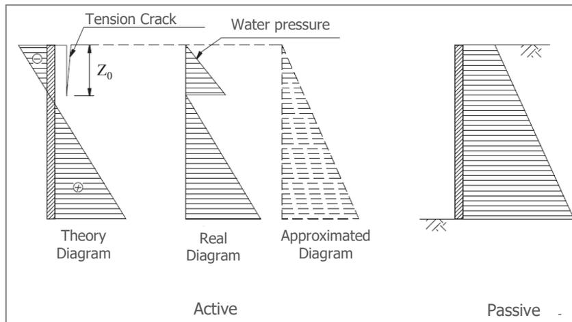
Figure 6 – Earth pressure distribution – Cohesive soil
