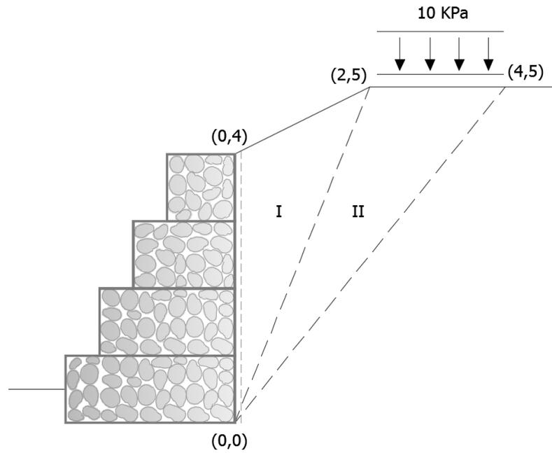
Figure 64 – Example 2 – Calculation of center of gravity
