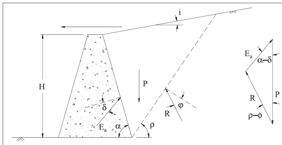
Figure 13 – Forces acting in the wedge – Active pressure
