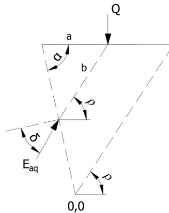
Figure 55 – Point of application – Load Active thrust
