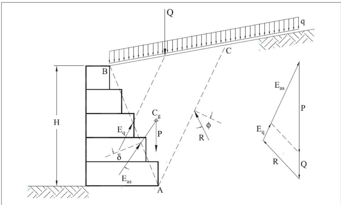
Figure 17 – Uniform load on the wedge
