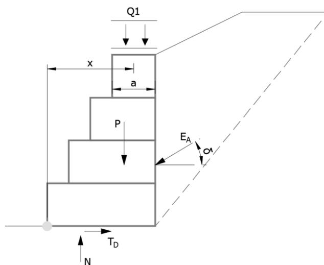
Figure 19 – Resistance moment due the load Q1
