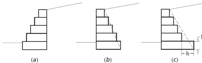
Figure 35 – Application surface of active thrust
