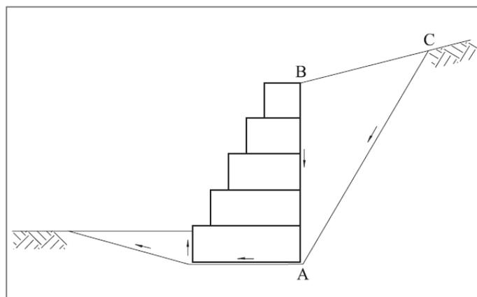
Figure 33 – Wedges considered in sliding analysis
