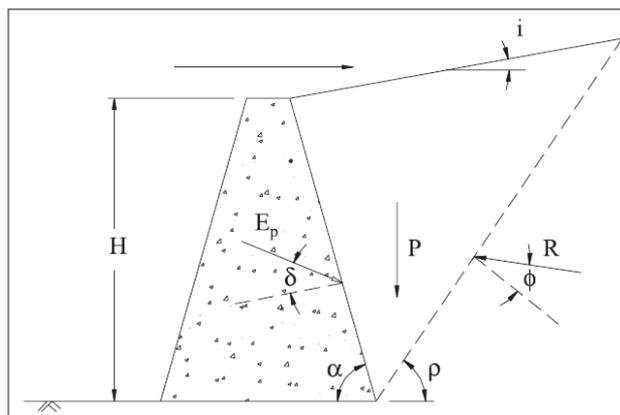
Figure 15 – Forces acting in the wedge – Passive pressure
