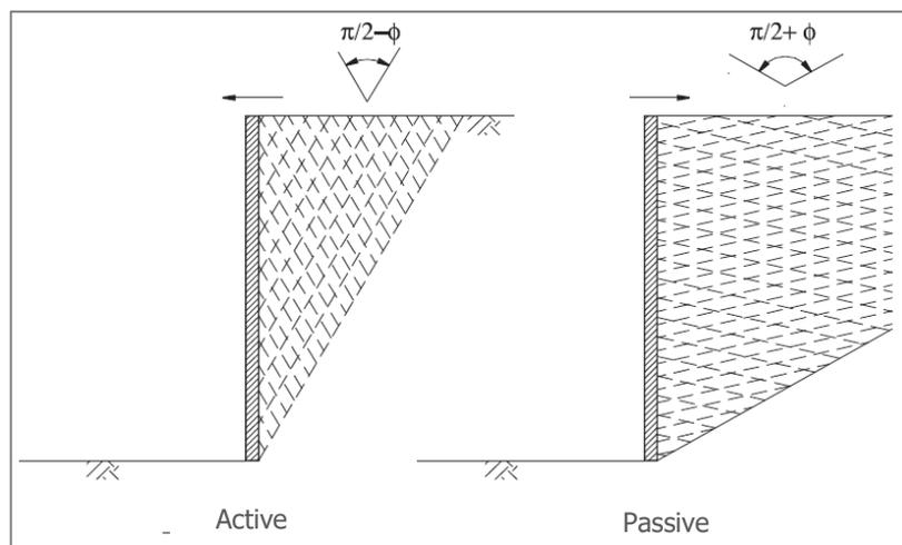
Figure 7 – Rupture plans in active and passive states
