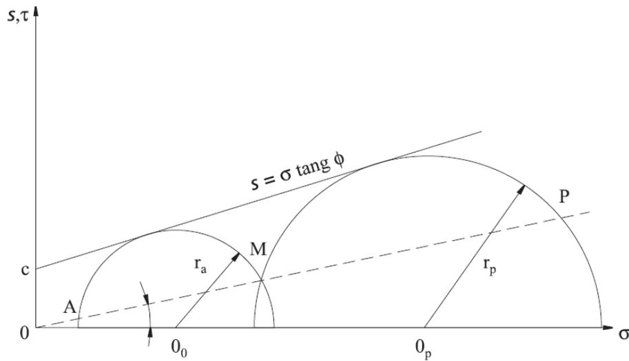
Figure 9 – Determination of horizontal pressures for cohesive soils
