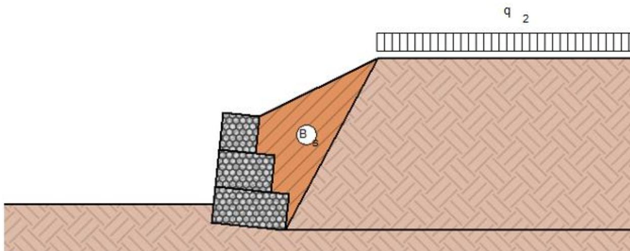
Figure 9 – Load Above Backfill – Q2
