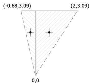
Figure 54 – Center of gravity of the wedge
