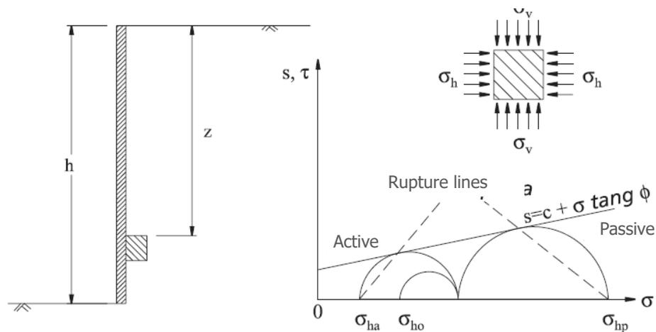
Figure 5 – Determination of lateral pressure
