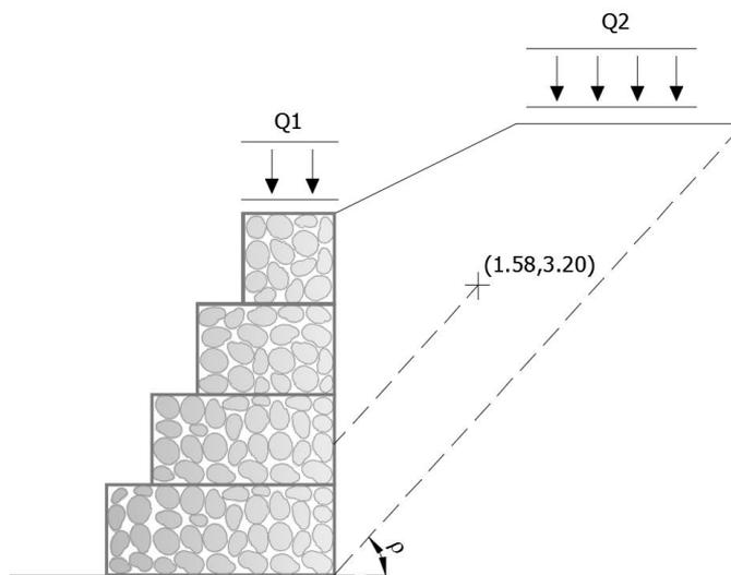
Figure 15 - Point of active thrust - Soil
