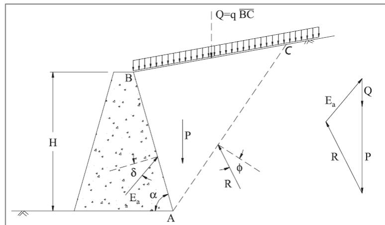
Figure 16 – Thrust due the uniform load
