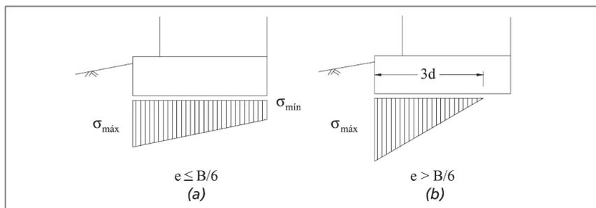
Figure 70 – Pressure distribution on base
