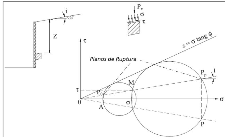
Figure 8 – Determination of earth pressure for  $i \neq 0$  ( $c=0$ )
