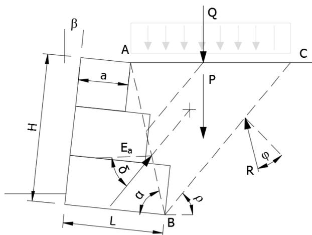
Figure 2 – Forces acting in the wedge
