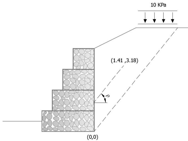
Figure 65 - Point of active thrust - Soil
