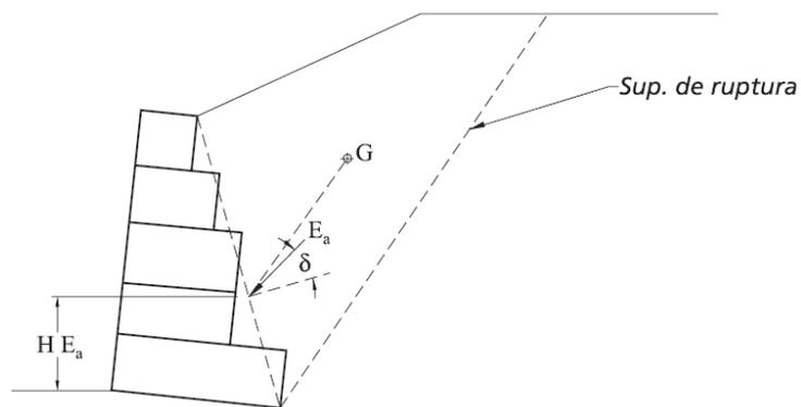
Figure 40 – Application point of Active Thrust
