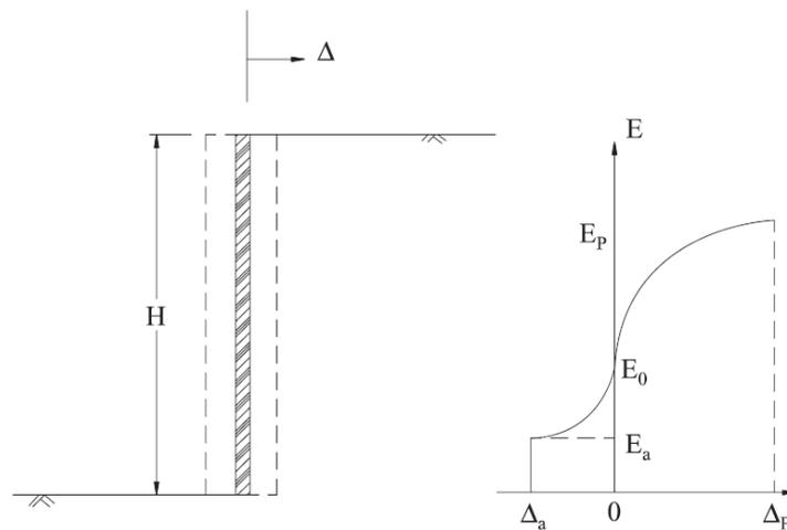
Figure 4 – Thrust over a bulkhead
