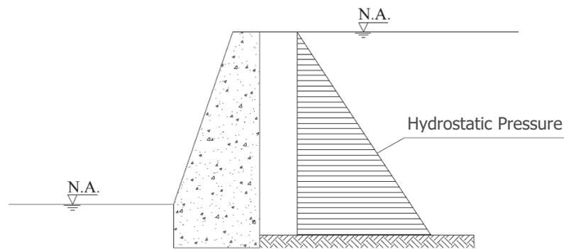
Figure 2 – Wall under hydrostatic pressure
