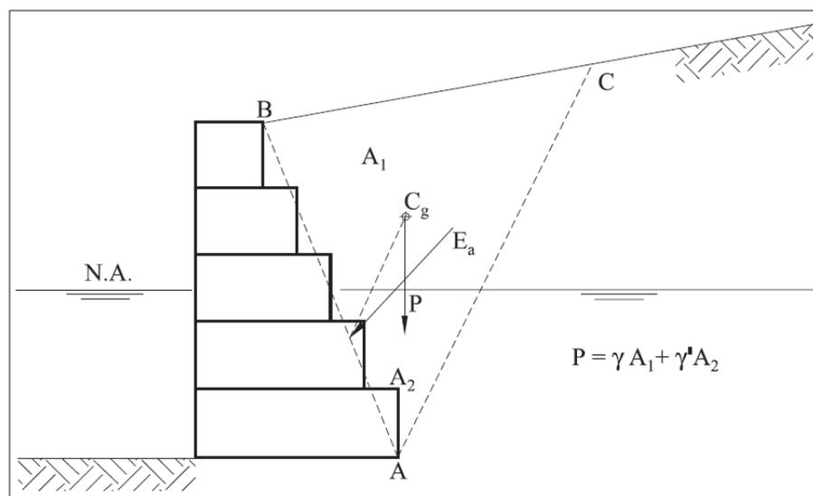
Figure 21 – Retaining wall partially submerged
