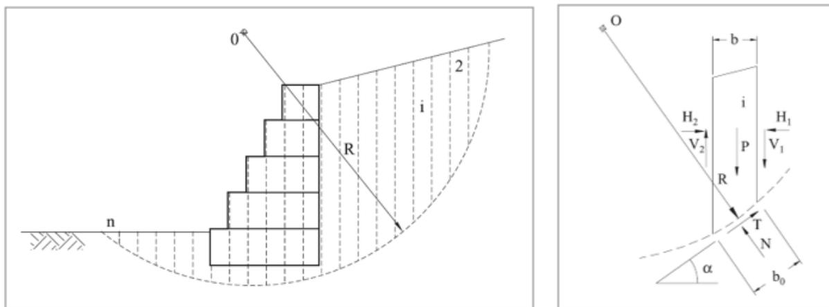
Figure 34 – (a) Bishop slice method (b) forces acting on slice
