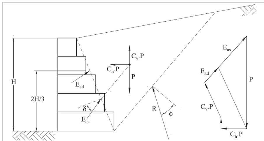
Figure 25 – Forces due the seismic consideration.
