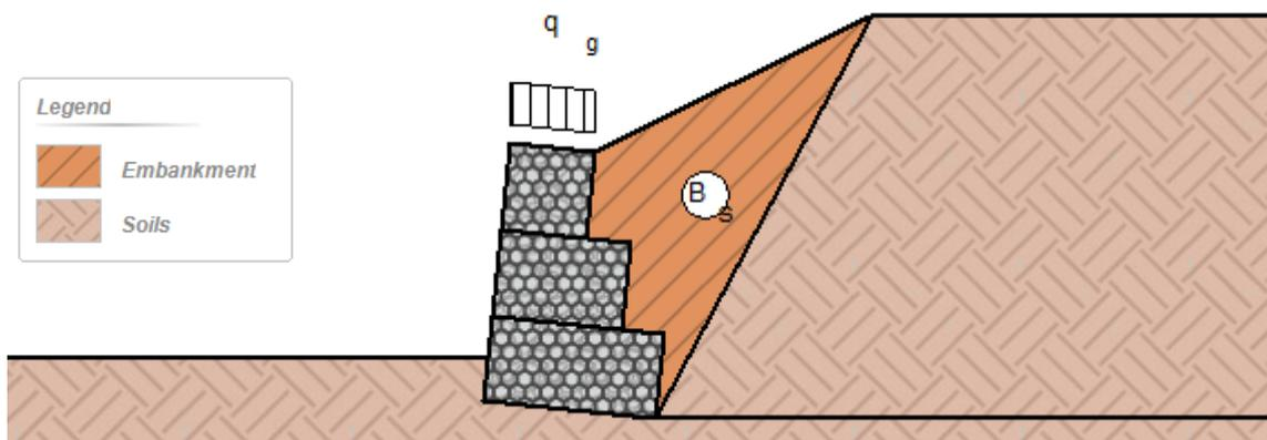
Figure 8 – Load above wall
