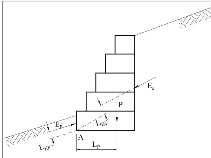
Figure 29 – Overturning check
