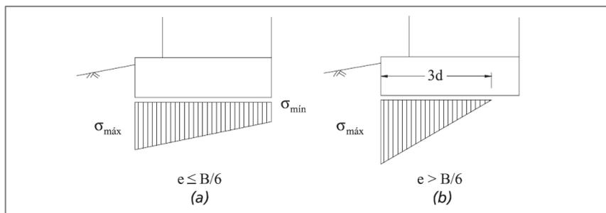
Figure 59 – Pressure distribution on base
