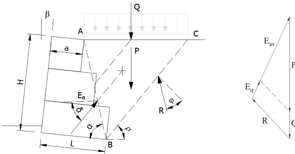
Figure 50 – Forces acting in the wedge
