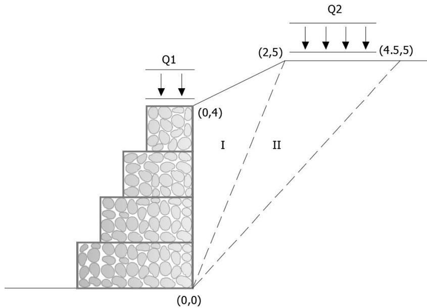
Figure 14 – Example 4 – Calculation of center of gravity
