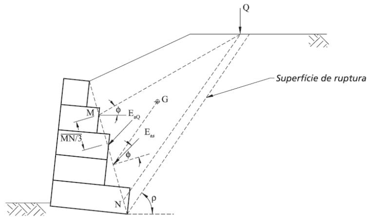
Figure 44 – Point of application of EAS and EAQ.
