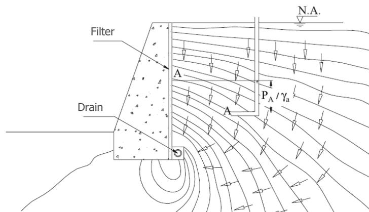
Figure 3 – Retaining wall with drainage system.
