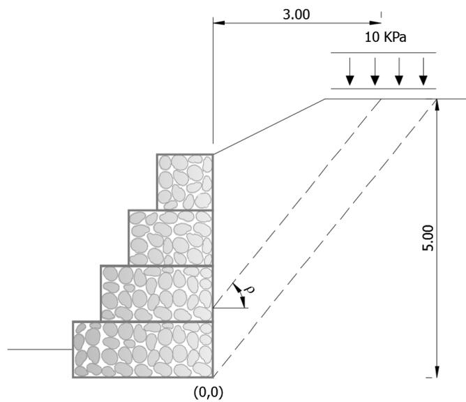
Figure 66 – Point of application – Load Active thrust
