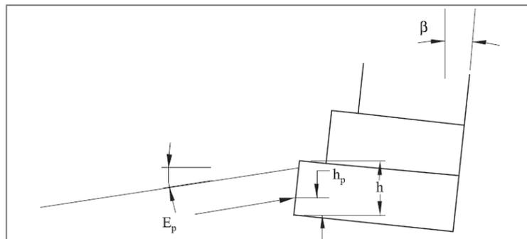
Figure 47 – Active Thrust Calculation
