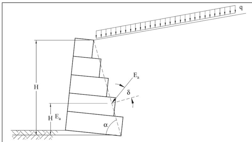
Figure 37 – Point of application – Active Thrust
