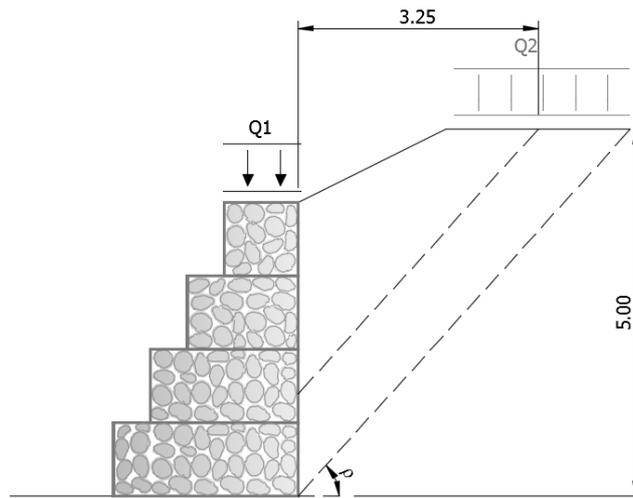
Figure 16 – Point of application – Load Active thrust
