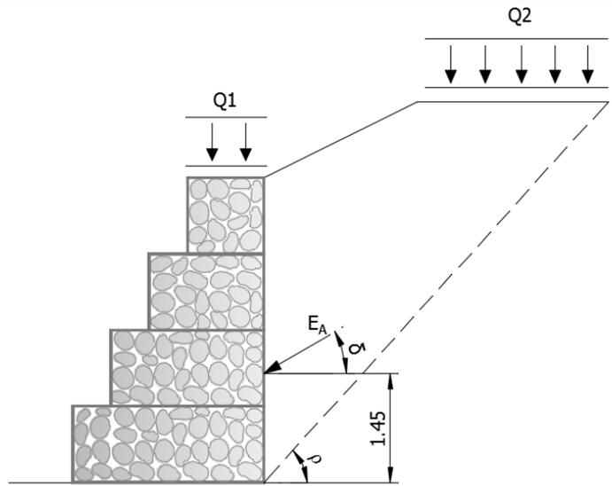
Figure 17 – Point of application | Active Thrust
