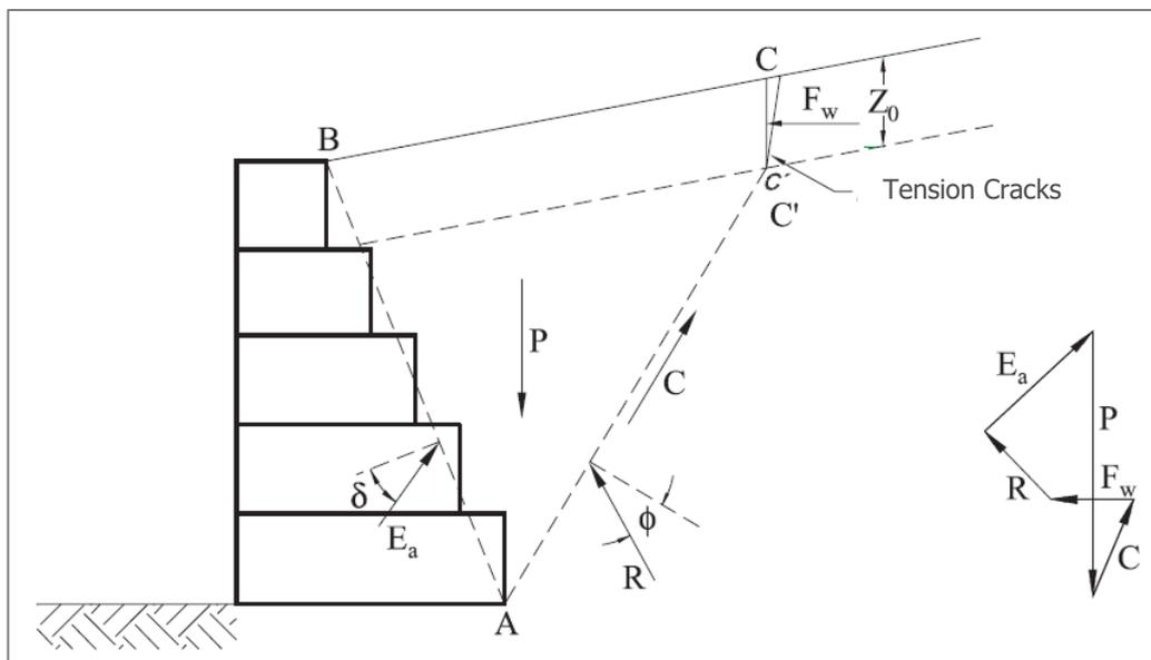
Figure 20 – Active Thrust – Cohesive soils
