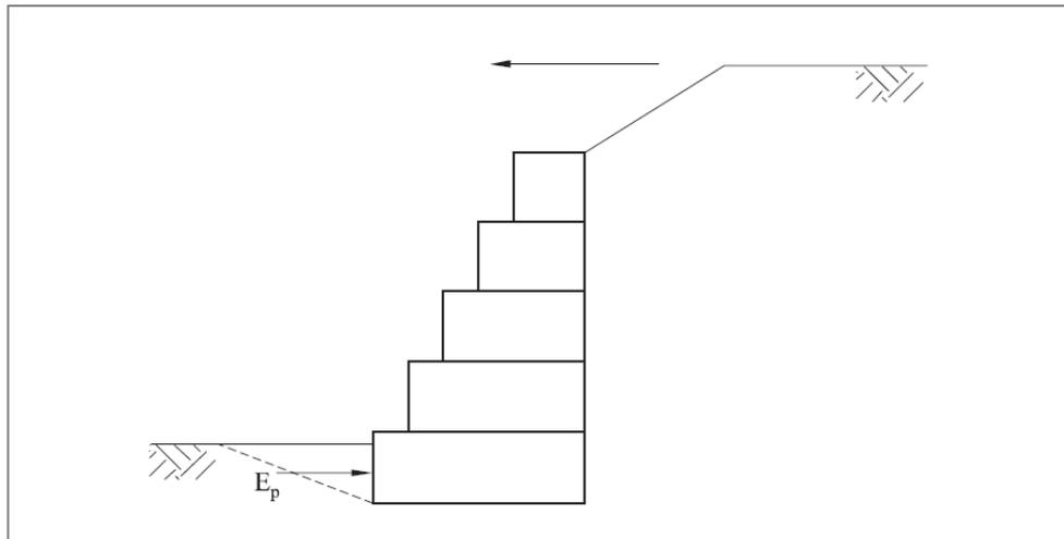
Figure 26 – Determination of passive thrust
