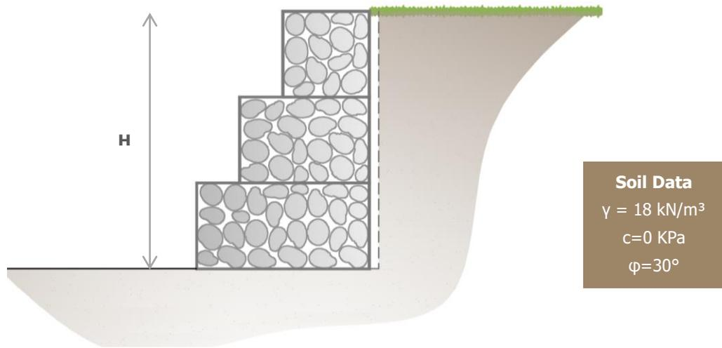
Figure 10 – Example 1 – Rankine Active Thrust
