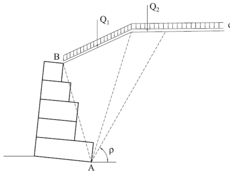
Figure 41 – Distributed load over backfill.
