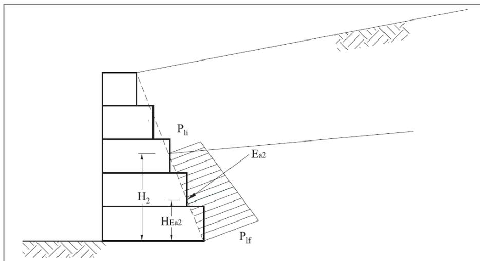
Figure 24 – Earth pressure distribution on the second layer
