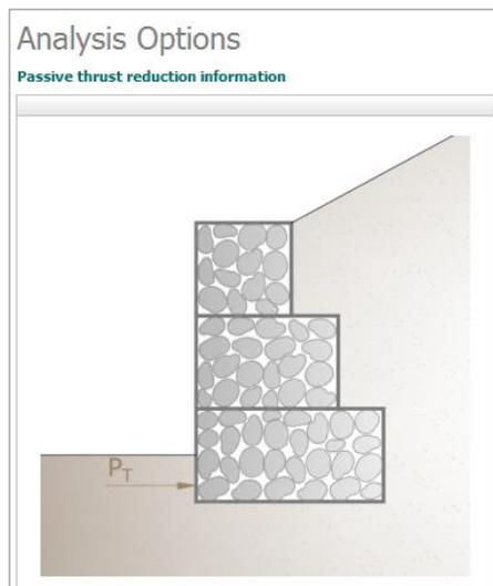
Figure 4 – Passive Thrust - GawacWin
