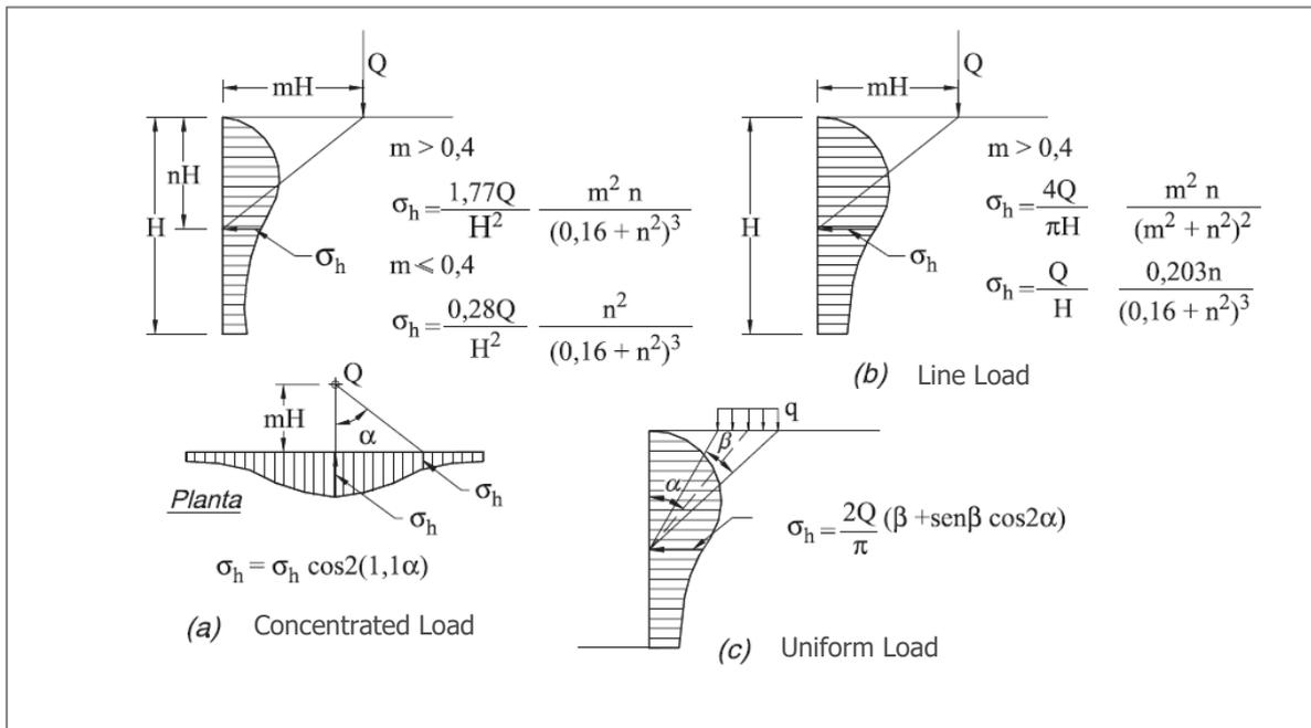
Figure 19 – Effects of surcharge by theory of elasticity
