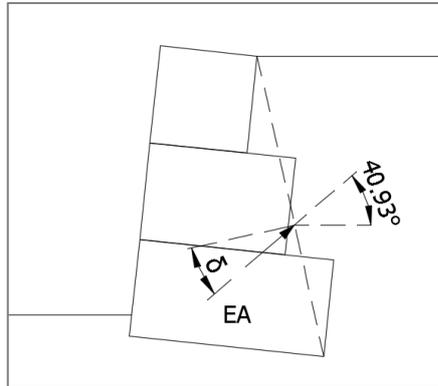
Figure 58 – Direction of active thrust
