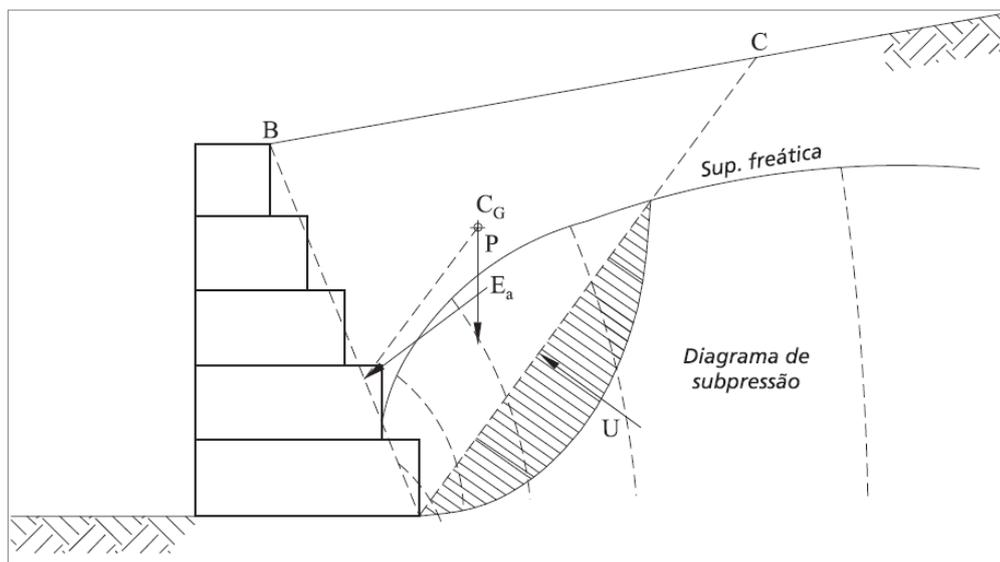
Figure 22 - Water percolation in the backfill
