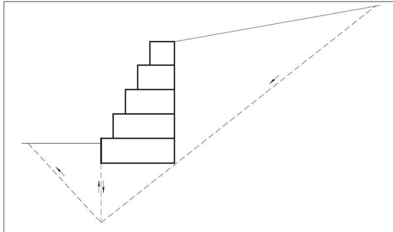
Figure 32 – Global stability analysis – wedge method
