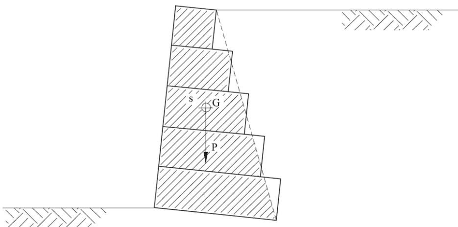
Figure 48 – Wall Weight Calculation
