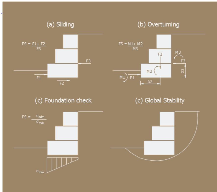
Figure 27 – Type of analysis – Gabion wall
