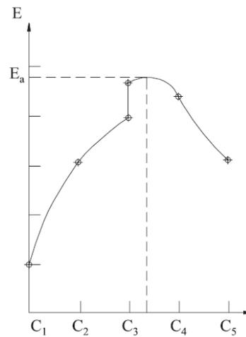
Figure 43 – Active Thrust variation due the inclination of failure surface.
