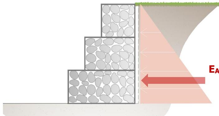
Figure 11 – Point of application of active thrust
