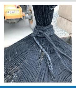
6. Lower the telehandler and remove the 8 loops. Attach the supplied metal lifting eye (O-ring) as shown in the images below.
