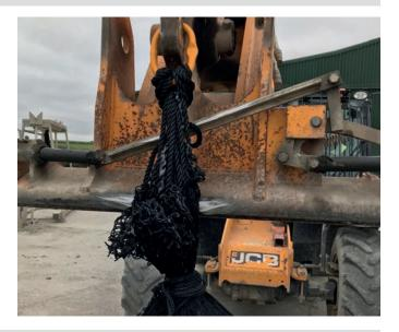
8. Put four appropriate chains into the hook of the telehandler and fix them properly to each corner of the frame and lift the frame carefully off the bag.
