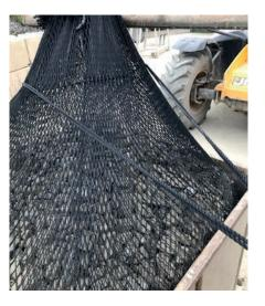
5. Lower the telehandler enough to loosen the tension on the 8 loops. Wrap the two ends of the tying rope around the top of the net in opposite directions and secure with a knot.
