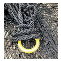
7. Place lifting eye in the middle of the telehandler hook and lift the AquaRockBag® to tighten the knot. Subsequently, lower the net and remove it from the telehandler.
